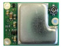
Figure 1-1 Jupiter Pico T GPS receiver (top view)
